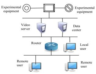
Figure 3. System structure of remote virtual training platform
