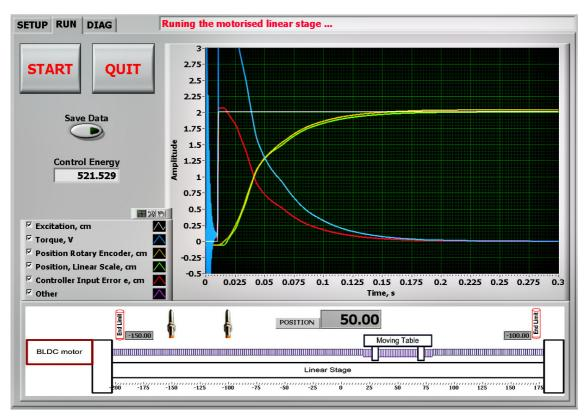
Figure 4. LabVIEW FPGA GUI for Execution of the Remote Experiment
