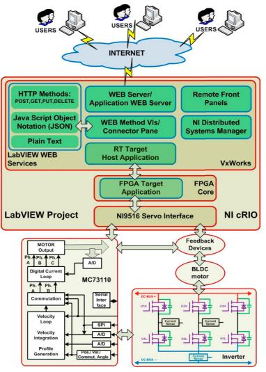
Figure 1. Architecture of the Remote Laboratory for Motion Control
