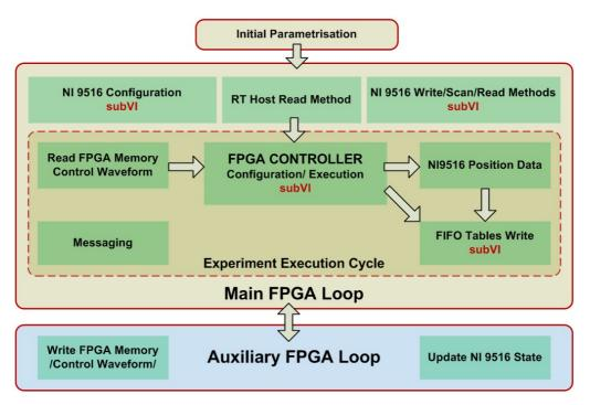
Figure 6. Functional Diagram of the FPGA Target
