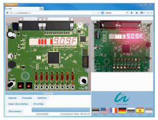
Figure 6. Web-interface of the rapid prototyping board (RIA)
