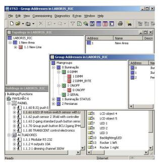
Figure 6. Configuration of the domotic system using the ETS software.
