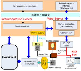
Figure 7. Implemented software architecture to control the KNX/EIB devices.
