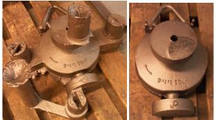
Figure 7. Example foundry workpieces. Left: before cutting. Right: after cutting.
