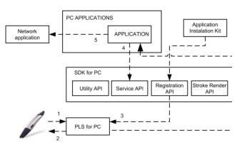
Figure 3. The PC architecture used by the digital pen [2]
