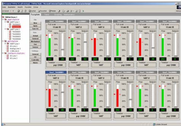
Figure 4. Web-based operating panel for 12 TMF instruments
