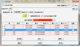
Figure 4. Machine limits set itinerary
