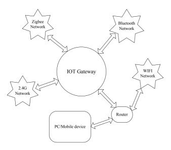
Figure 1. Architecture of IOT gateway in the experimental platform
