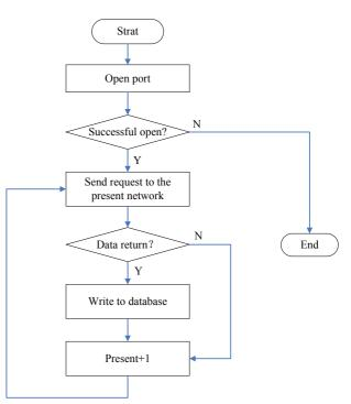
Figure 2. IOT gateway data transmission control
