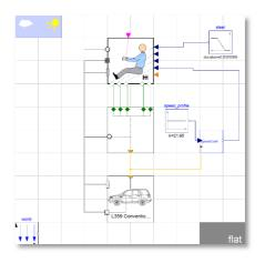
Figure 3. Vehicle model interface with driver model
