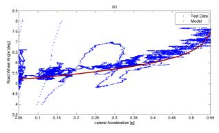
Figure 8. Steering response, real data vs. model
