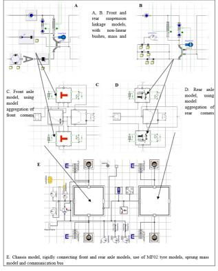
Figure 2. Vehicle model construction
