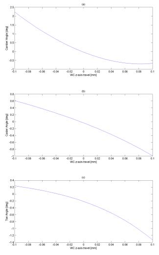
Figure 7. Caster camber and toe curves from model based rig
