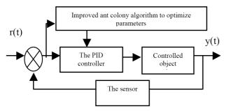
Figure 3. The principle diagram of the control program of improved ant colony algorithm
