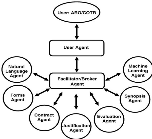
Figure 1. Agent architecture and communication channels.
