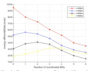
Figure 3. The comparison of energy efficiency for different radius of user location with k = 1.
