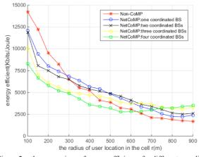
Figure 2. the comparison of energy efficiency for different coordinated BSs with k = 1.
