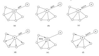
Figure 7. SPIN protocol routing establishment and data transmission
