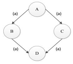
Figure 2. Flooding protocol implosion
