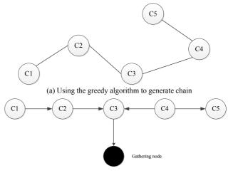
(b) The path of the data transmission to the gathering node Figure 6. PEGASIS protocol
