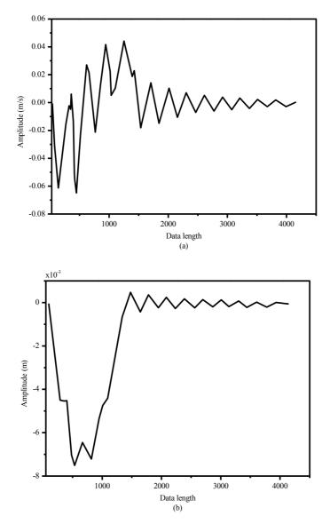
Fig.5. Speed (a), displacement (b) signal waveform based on acceleration signal
