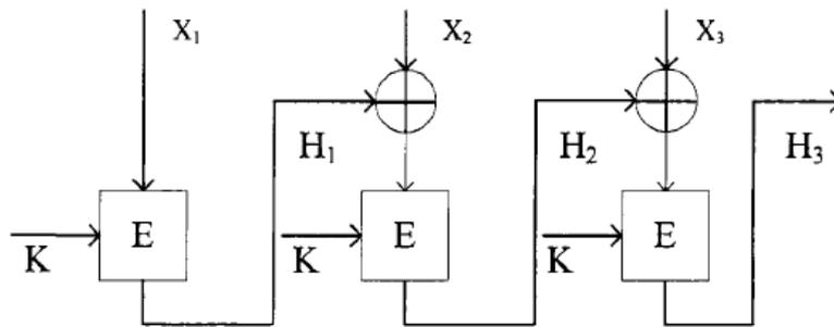
Fig. 4. Message authentication code calculation
