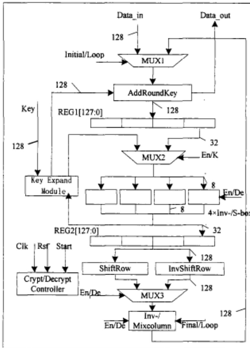
Fig. 1. AES encryption and decryption data path
