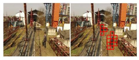
(a) 317th frame (b) Motion target marking
