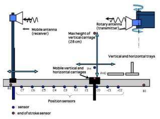
Figure 4. Sketch of the antenna workbench and its different elements and sensors.
