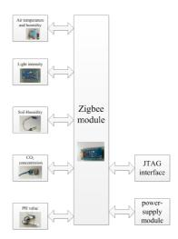
Fig. 4. Hardware structure diagram of the system
