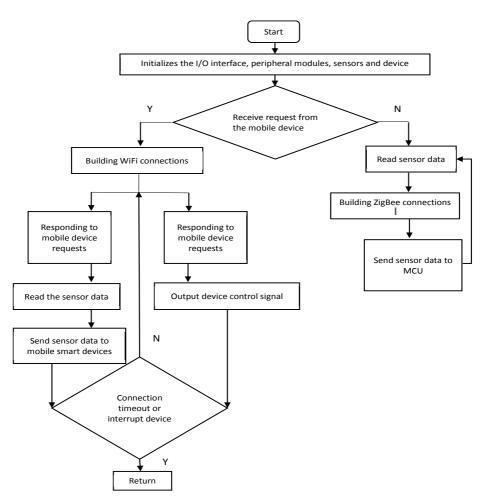
Fig. 3. Workflow diagram of the system
