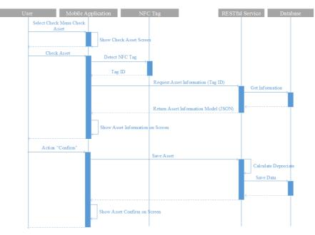
Fig. 3. Sequence Diagram: ASCMS-Based monitoring asset
