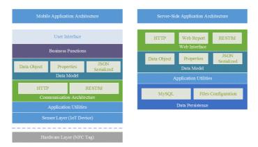
Fig. 4. Mobile and Server-Side Application Architecture of ASCMS
