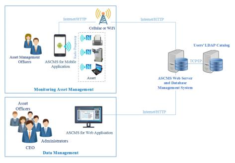
Fig. 2. IoT Process Diagram of ASCMS
