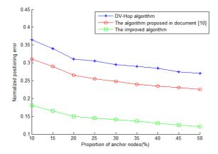
Fig. 5. Relationship between the proportion of anchor nodes and positioning error
