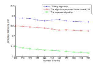
Fig. 6. Relationship between the number of nodes and positioning error
