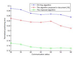
Fig. 7. Relationship between communication radius and normalized positioning error
