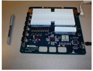
Figure 2. The Digital Electronics FPGA Board used in stand-alone mode
