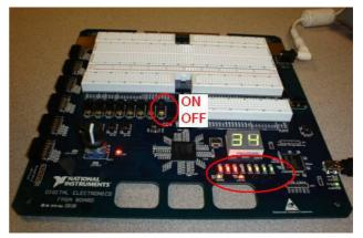
Figure 8. LEDs and SW0 on the Digital Electronics FPGA Board
