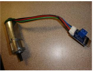
Figure 12. PmodHB5 module with motor attached
