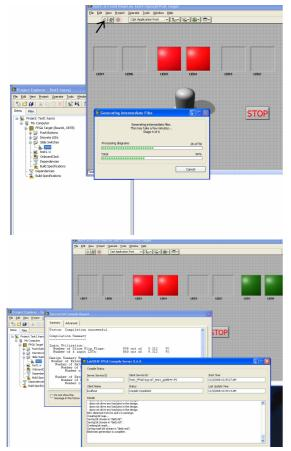
Figure 11. LabVIEW FPGA VI compilation
