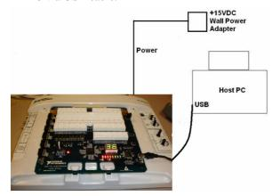
Figure 4. The Digital Electronics FPGA Board used in NI-Elvis mode
