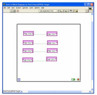
Figure 7. LabVIEW FPGA diagram using FPGA I/O objects
