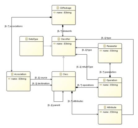
Fig. 2. The simplified class diagram metamodel
