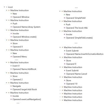
Fig. 6. IFVM bytecode result of compilation unit
